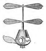
This revolving of the propellers in opposite directions keeps the car from gyration.
